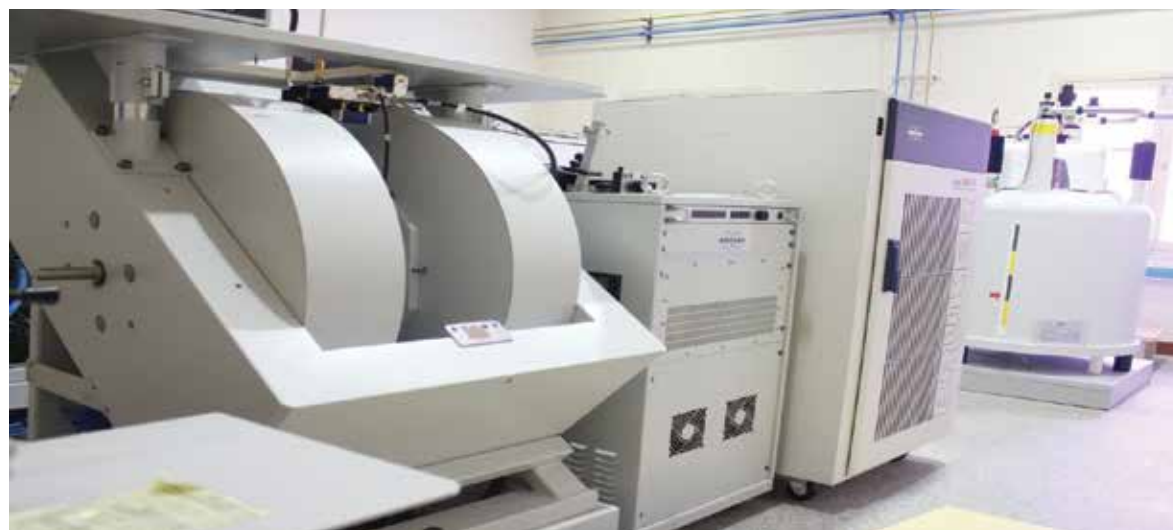
Figure 50. Top view of part of the custom-built multi-band DNP system: (l to r) X/Q-band electroma.
